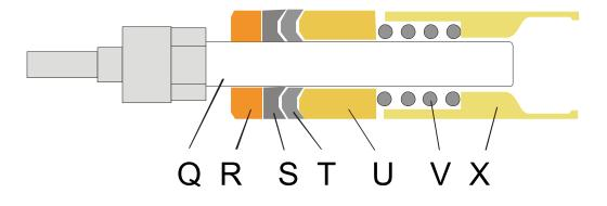
Unscrew the big retainer nut Y3 at the back of the cylinder Y 5. Remove cooling plate Y 2. Gently knock out all the internal parts in the cylinder R until X. Inspect the wear parts R, S and T replace if necessary.
