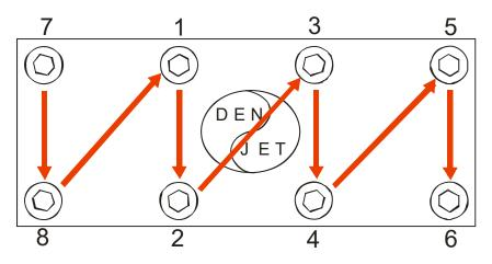
Tighten the bolts in the above shown pattern in steps of torque. (20Nm - 100Nm - and finally 200Nm) alternating between bolts
