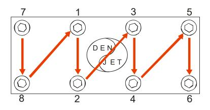
Do not loosen one bolt entirely, loosen them bit by bit and alternate according to the pattern. Pull out the valve by applying pressure in the extraction groove with 2 flat-face screwdrivers as shown below:
