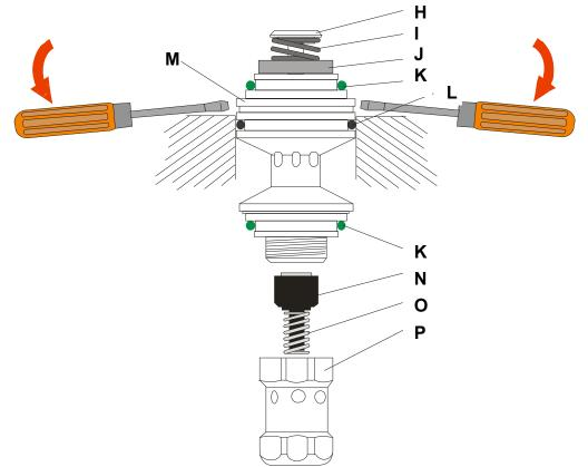
Dismantle the valve assembly by clamping on the spanner face of the valve-body M And unscrewing H and P.
