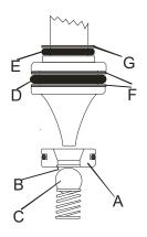
Re-adjust the safety valve by running the machine with a correctly sized nozzle. Pull the trigger and start tighten the nut for the thick black spring, until there is no leak from the safety valve.
