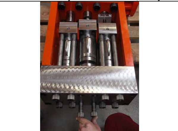
Unscrew the 2 upper bolts entirely, loosen but leave the bottom bolts engaged.
