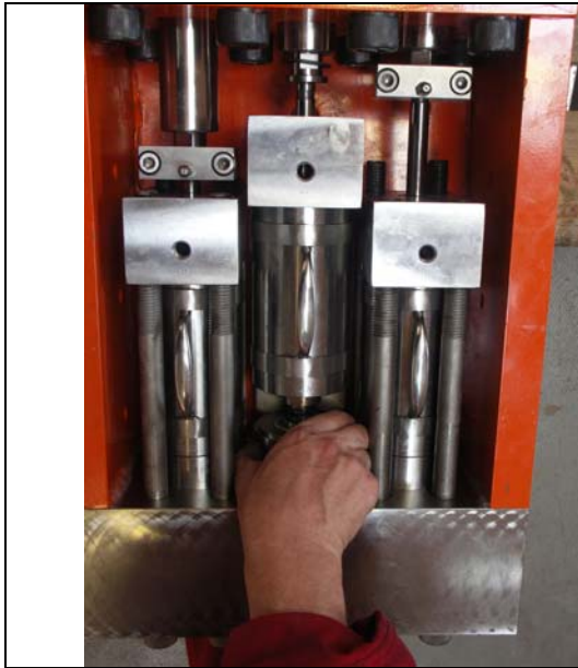
Slide out valve cartridge.
