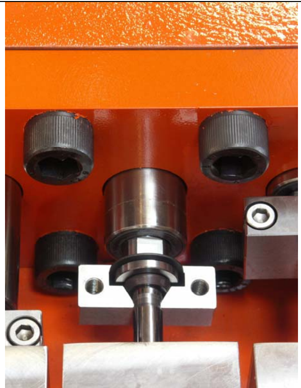
Take off floating plunger holder, take care of small pieces.
