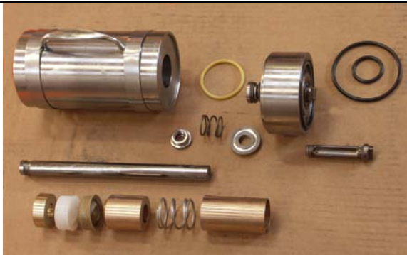
Slide out valve cartridge.
