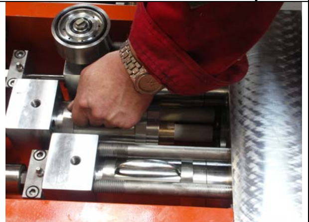
After changing worn parts, slide back stuffed cylinder.
