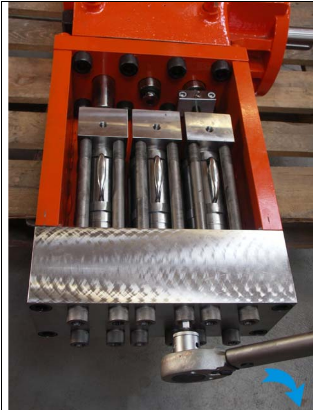
Tighten cylinder head screws in an alternating manner to 450Nm.
