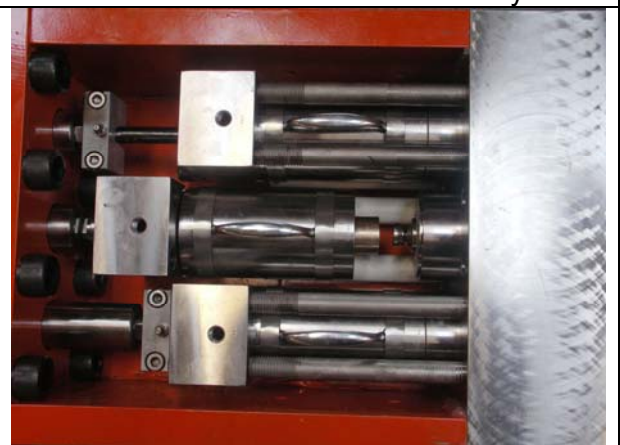
Align cylinder and valve to back block and manifold recess.
