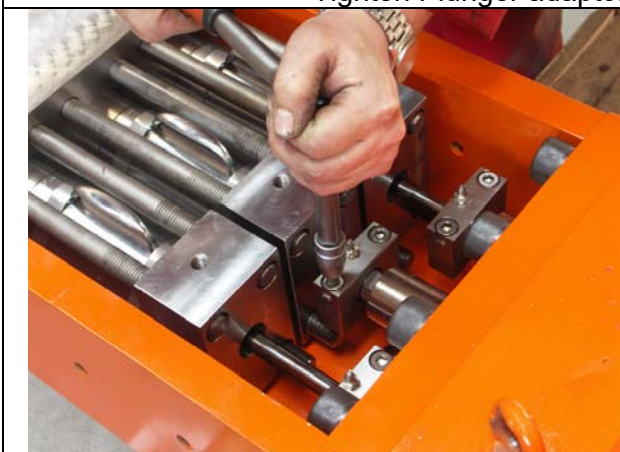
Tighten floating plunger clamp.
