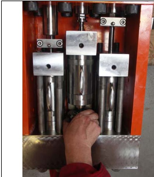
Slide out valve cartridge.
