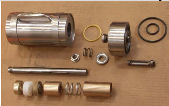
Slide out valve cartridge.
