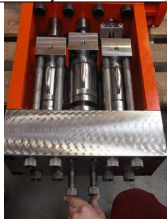
Unscrew the 2 upper bolts entirely, loosen but leave the bottom bolts engaged.
